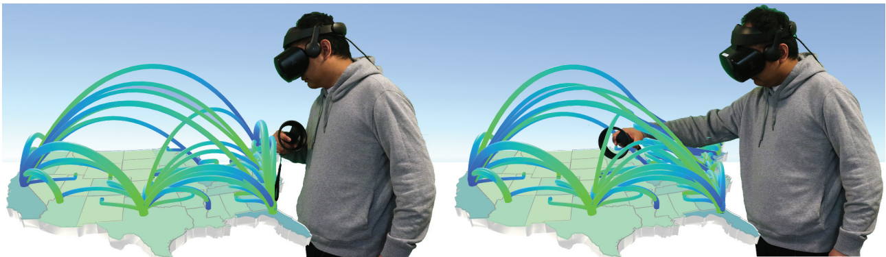
Figure 10. User pushing away a map symbol to reveal hidden information. Left: A thick and long flow starting in Florida and ending in the northeastern U.S. hides shorter and thinner flows. Right: The user is pushing the long flow away with the controller to reveal the smaller flows.
