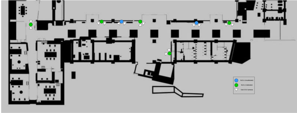
Figure 7: Top-Down Map of Infrastructure Cameras in Experimental Setup
