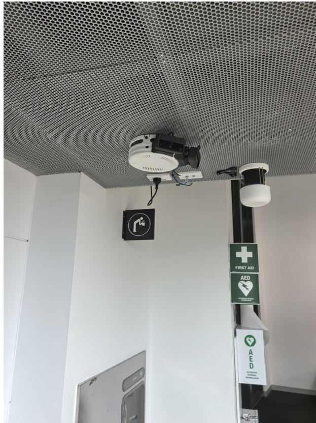
Figure 14: Physical deployment of the OAK-D S2 stereo-vision camera mounted within the Monash Innovation Lab. This hardware formed the visual foundation of the distributed edge network.
